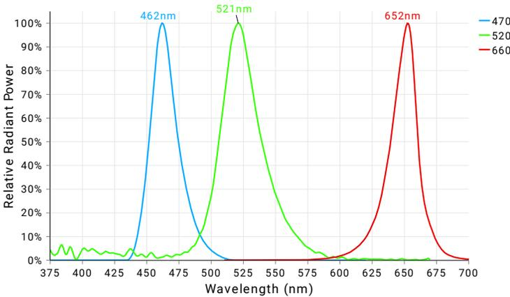
Visible color illumination consists of using wavelengths between 400-700 nm to either create or eliminate contrast on an inspection subject based on differences in a features color hue. When referring to a color wheel, simply remember the following; like colors reflect and brighten surfaces; conversely, opposing colors absorb and darken surfaces.
