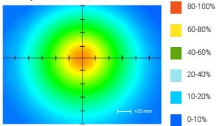
Optical measurement taken using SL147-WHIIC Rev. A @ 300 mm
