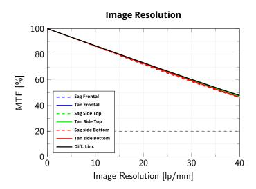
Modulation Transfer Function (MTF) vs. Image Resolution, wavelength range 486 nm - 656 nm at wf/16 of cylindrical object of diameter 25 mm and height of 17 mm
