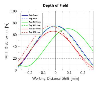
Modulation Transfer Function (MTF) @ 20 lp/mm vs. Working Distance Shift from the best focus Working Distance, wavelength range 486 nm - 656 nm
