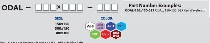
The 5-pin M12 connector is located on the width side of th light. Sizes listed are in millimeters.
