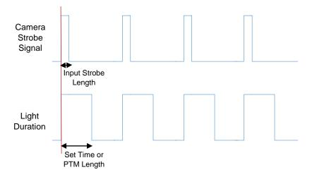
Light Duration is determined by the selectable set time on the PTM and does NOT depend the camera strobe signal. Light triggers on rising edge of strobe pulse.
