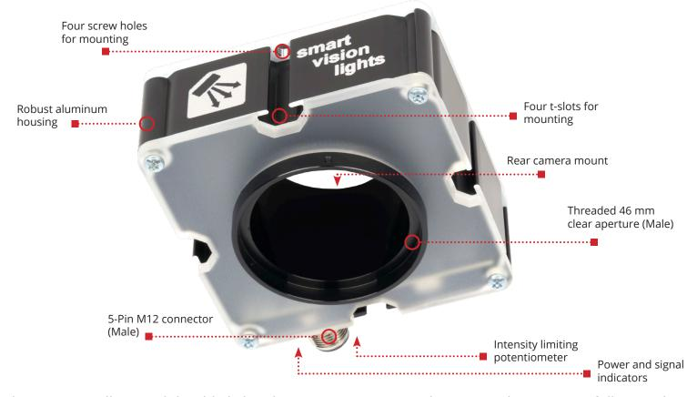
The R80 is an all-around durable light. The 10%-100% intensity limit control gives users full control over light output. A standard 42 mm inner hole diameter allows for use with nearly all camera systems with available step-up and step-down conversion kit adapters.
