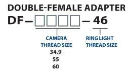
\*When mounting an EZ Mount Ring Light, a double-female adapter is used.
